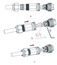
Fig 6.2 AC output wiring diagram
