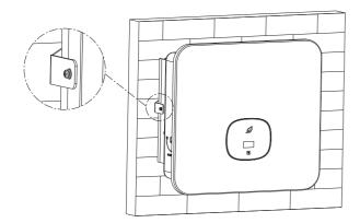
Fig 5.9 Schematic diagram of inverter wall mounting
