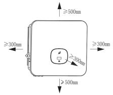
Fig 5.2 Installation dimensions for one inverter
