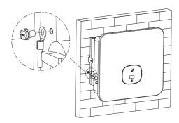
Fig 6.1 Grounding diagram
