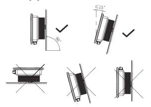
Fig 5.1 Installation diagram
