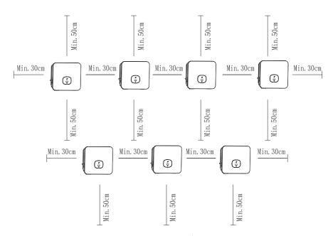
Fig 5.3 Installation dimensions for multiple inverters
