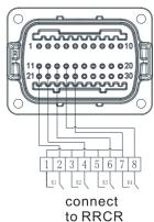
Fig 6.17 Inverter – RRCR Connection
