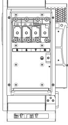
2>Determine the stripping length (approximately 30mm) according to the specifications of the crimping terminal. Use crimping tools to crimp the wires and terminals, then connect the cables to the corresponding channels through the waterproof interface, and tighten the screws.
