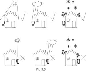
B. To reduce the de-rate performance of the inverter and extend inverter's life span, we strongly recommend you install an awning, for the distance between an awning and inverter, please refer to following drawing.
