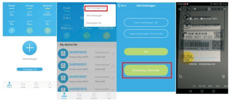
2>User can add datalogger at the datalogger list page to add a datalogger, edit, delete, configure etc.
