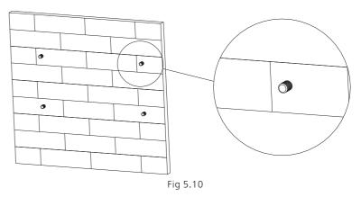
Notice: Expansion bolt should be installed on solid walls with at least 100mm thickness. 2>Follow the following drawing put the bolt to install the wall mount plate on the wall.
