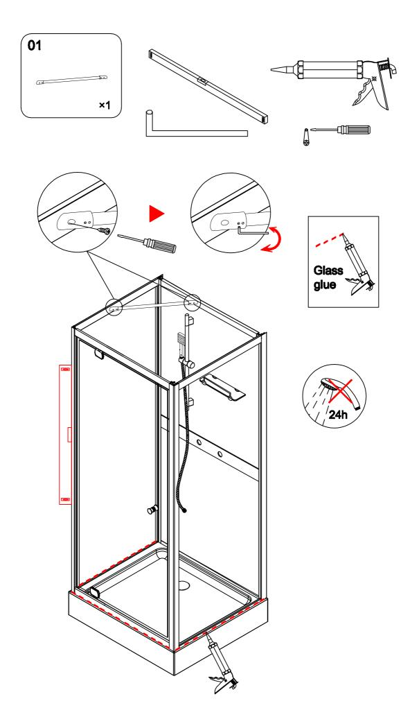
Before the final set up of this shower enclosure, check its watertightness. In case of leakage, retighten the screws and if necessary add silicone. Caution: Please handle all glass with care. Any damage to the edges or scratches to the surface that occur during assembly or normal use can cause the glass to break suddenly. Tempered glass will shatter into very small pieces that will still have sharp edges.
